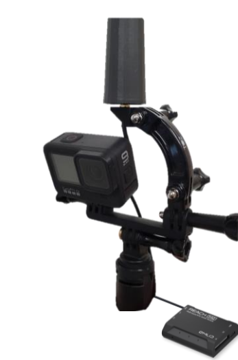
An Emlid Reach M2 RTK GNSS unit paired with a GoPro Hero9.
