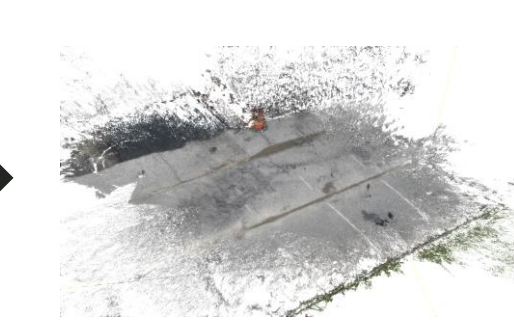
Reconstruction of pavement using Pix4D.
